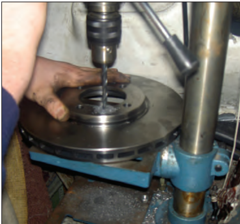
Accurate drilling of Capri vented disk after being accurately marked.
