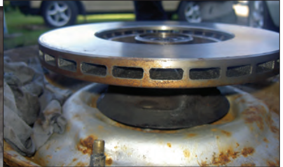
New Disk bolted to hub. I use an old wheel rim as a stand
